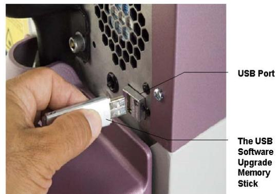
Figure 6.1: Laser System Software Upgrade USB Port and Memory Stick
