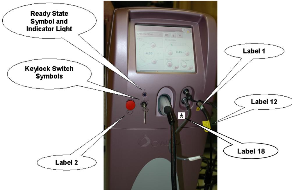
Figure 7.3: Control Panel and Delivery System Label Locations
