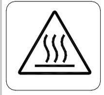
**Label 6 and 7: Heat or Hot Surface Warning Label applies when unit is powered and/or after it is turned off.**
