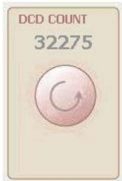
The Canister Count parameter indicates the total number of DCD Spray pulses remaining in the cryogen canister for the selected spray duration. The counter accuracy depends on the user pressing the reset button with the circular arrow on it after installing a new DCD canister. It is present to give the user an indication of the canister’s relative fill status.
