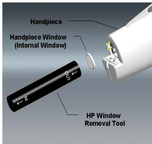
Figure 6.4: Handpiece Window and Removal Tool
