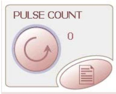
The Treatment Pulse Counter parameter on the Main Screen (Figure 3.2) indicates the number of times the laser has been pulsed. This counter can be used to keep track of the total number of laser pulses used in a treatment session.
