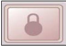
A password protected Software Lock is included to prevent unauthorized use of the laser. The laser will remain in warm-up mode when the software lock is engaged. The software lock will be initiated by the user. When the Screen Lock Button is pressed on the Main Screen Menu (Figure 3.2), it will query the user about locking the screen.
