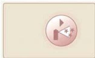
The Purge Button is used to remove air bubbles from the DCD cryogen line when a new canister is placed in the system or a handpiece is installed. This action must be done with the handpiece removed from the calibration port and pointed in a safe direction. When pressed, the handpiece will disperse cryogen spray for the selected spray duration. If the button is held for longer than 1 second, a short spray and then a longer spray of cryogen (up to 3 seconds) will be dispersed.
