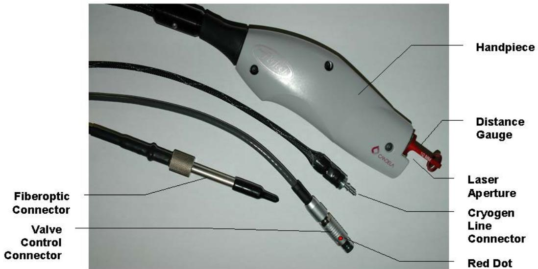
**Figure 6.9 Handpiece Delivery System Close-Up**
