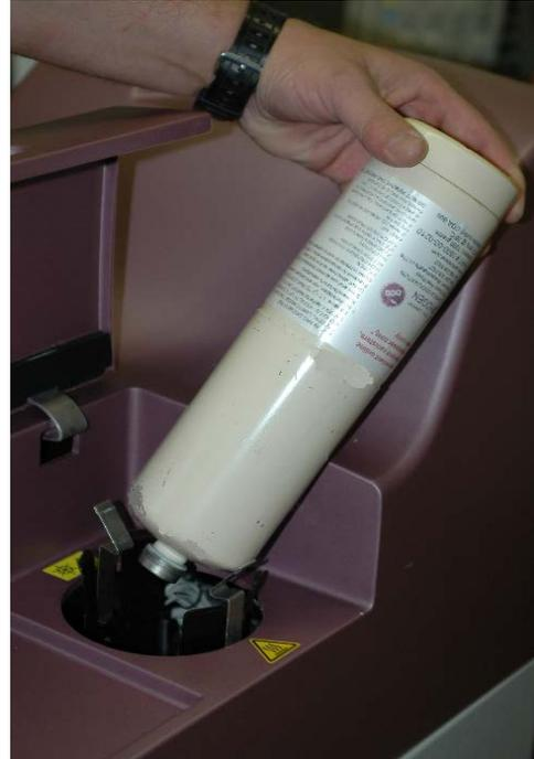
**Figure 6.11: Cryogen Canister Replacement**
