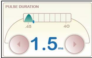
The Pulse Duration parameter is the duration of the pulse delivered to the patient and can be set to between 0.45 – 40 milliseconds. To ensure that the selected fluence is delivered, the laser will automatically require that a calibration procedure be performed anytime the Pulse Duration parameter is adjusted.
