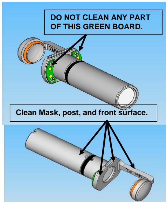
Figure 6.6: PL Distance Gauge Cleaning
