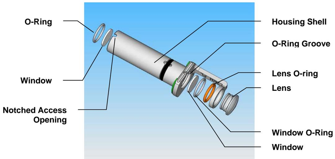
Figure 6.3: Pigmented Lesion Distance Gauge Windows and Lens
