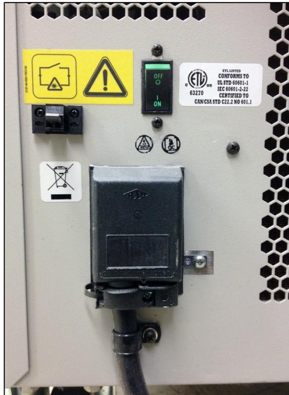
**Figure 1.7: Replaceable Power Cable Inlet Attachment**
