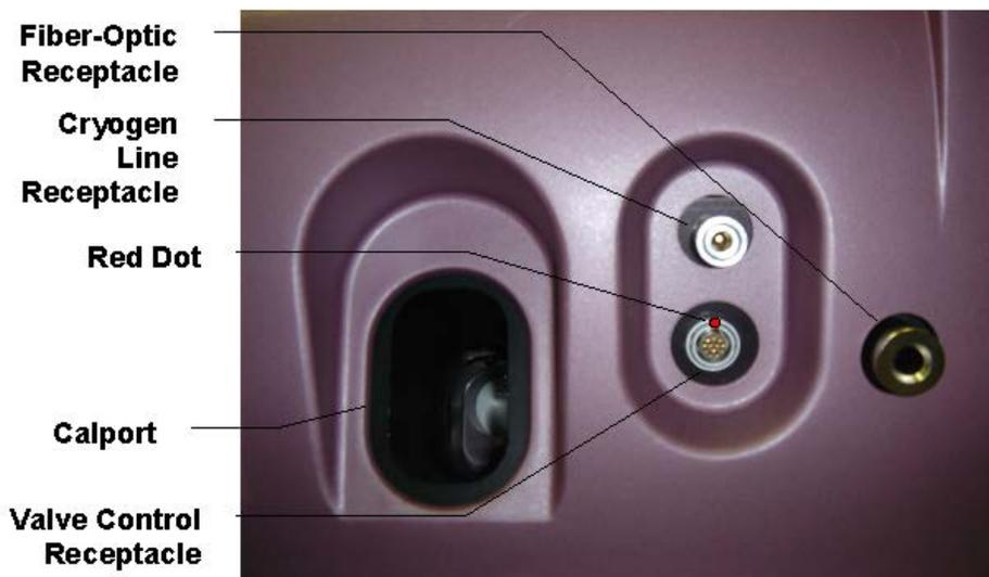
**Figure 6.10: Control Panel Close-up of Delivery System Receptacles**
