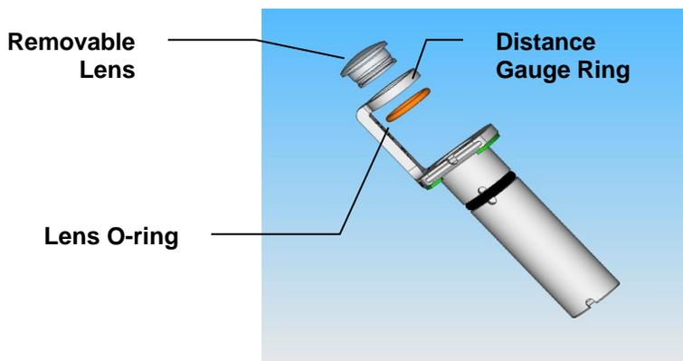
Figure 6.7: PL Distance Gauge Lens
